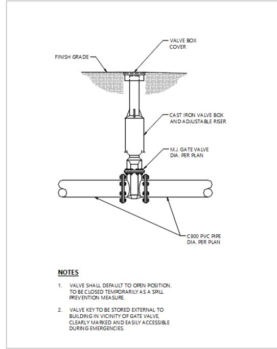
**Drainage Emergency Shutoff Valve**
